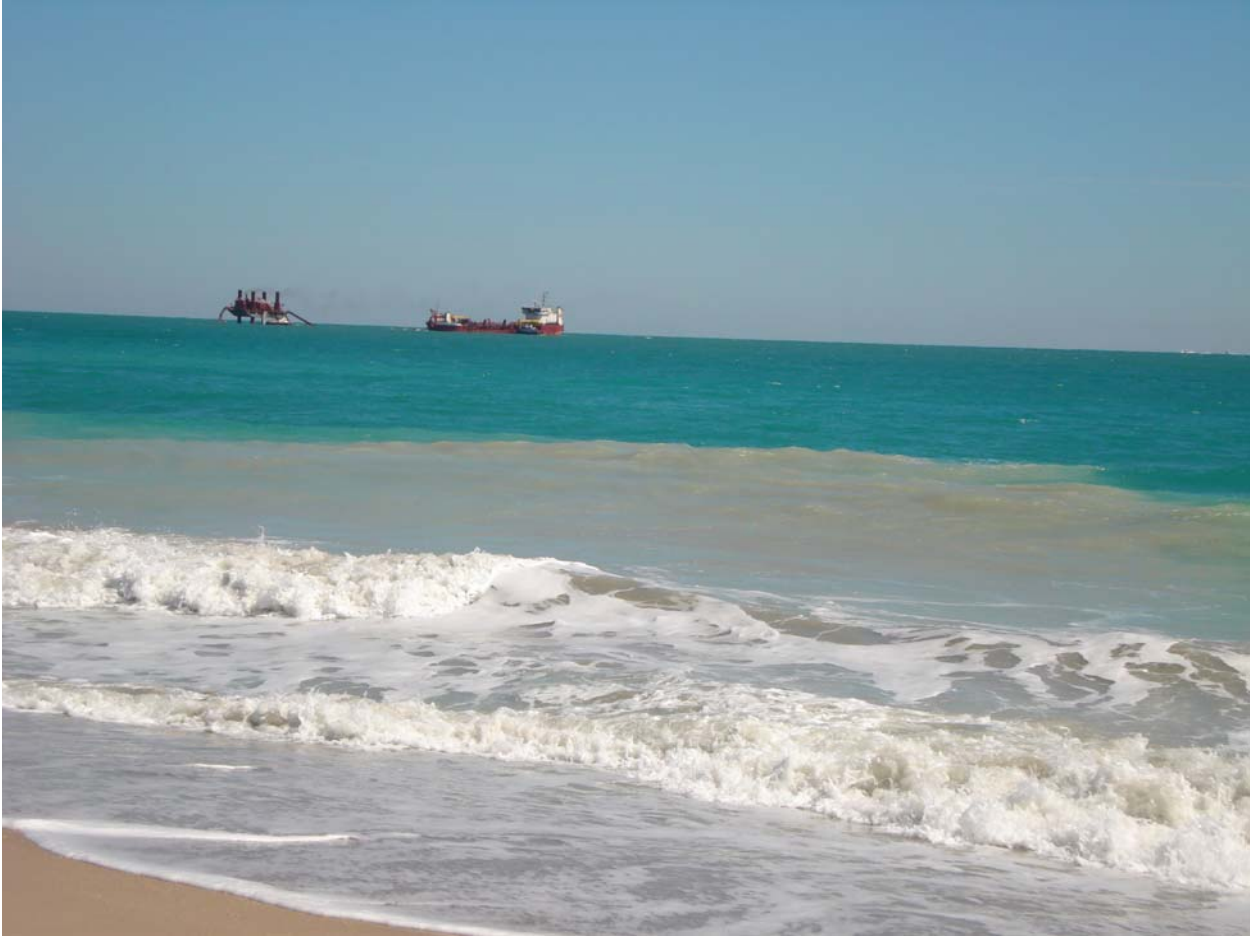
Figure 6. Hopper Dredge and Pumpout Booster. The pumpout hook-up is located in the nearshore in water depths sufficient to allow the dredge to hook to the discharge pipe. In this case a booster pump on a jack-up barge is utilized to extend the range of the pumpout discharge. This dredge ( The Dodge Island ) has a hopper capacity of 3,600 cubic yards. Active pumpout is occurring within the photo. Note the presence of turbidity within the immediate nearshore.
