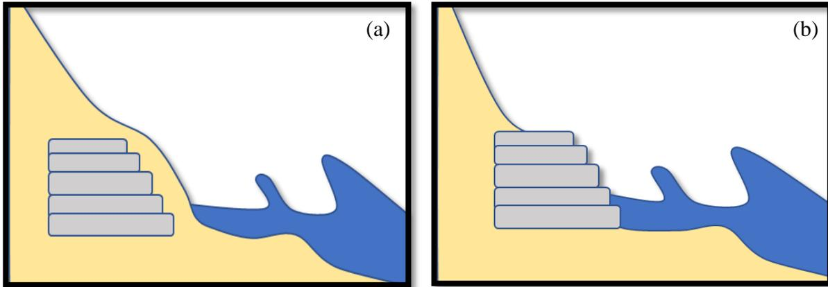
Figure 1 Schematic profile view of the geotubes (a) before the exposure of the geotubes. In this case, sediment is still available for the natural erosion. Once the geotubes are exposed (b), the littoral system receives a reduced sediment load.
